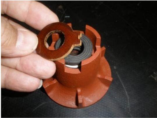
Prior to heating up the impeller for installation we took a look at the seal and seal spring and the position we are looking at prior to installing on the water pump
