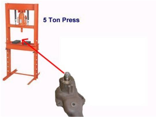
Place you water pump in the 5 ton press and push the bearing shaft out the cast iron water pump casing. Also use your press to push out the bearing shaft from the impeller.
