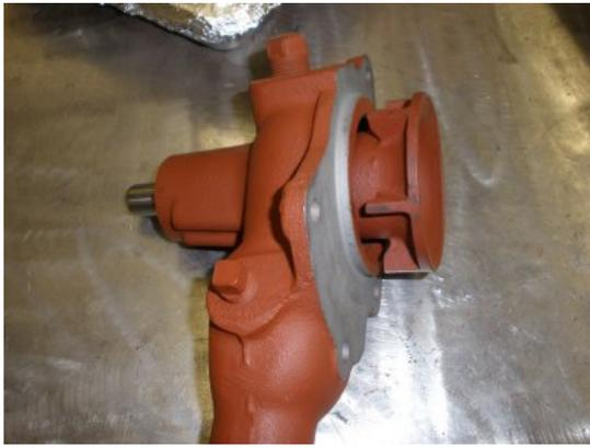
Terrific! the impeller should be pushed to the end of the shaft as directed by the TM.
