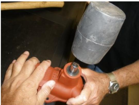
After the primer dried, Note: the TM shows to use the press to push the bearing shaft into position. We heated the casing up to about 250 degrees for about 30 minutes and took the bearing shaft and gently tapped it in with a rubber mallot, being carefull not to damage the water sealed bearing.
