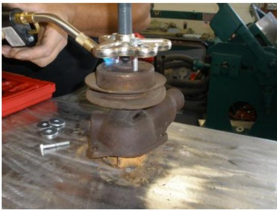
We start by screwing in the pulley puller onto the pulley. Here we use a modern pulley, and heat the pulley just before we start to rotate the pulley bolt to remove the pulley.
