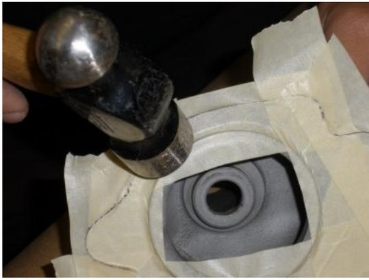
Before we press the bearing shaft we are going to primer the casing. Here we tape the surface area to protect where the gasket will be applied. Tip: use a hammer and tap on the edges and the excess tape will tear right off for a clean protection area.
