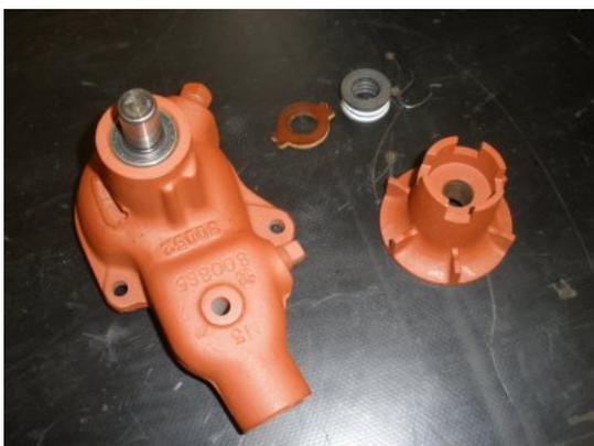
After the bearing shaft has been installed with a press into the casing, we are now ready to press fit the impeller to the back of the shaft. After checking the measurements, and the impeller only a couple thousands dimension different, we decided to head the impeller an push it on gently. Note, you want to be careful not to damage the bearing shaft by not pounding on the impeller.
