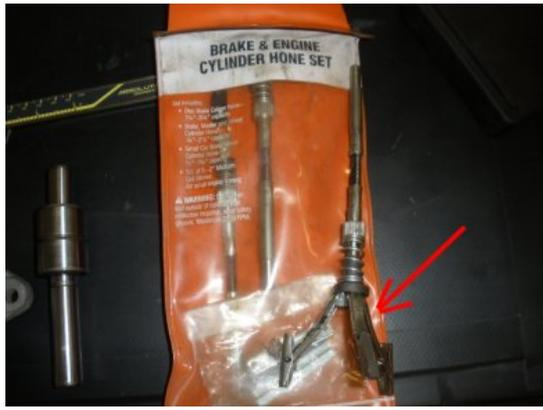
We measured the diameter of the new bearing shaft and the inside diameter of the water pump and decided to hone (smooth) the inside of the water pump. Here used and Engine Honeing kit.
