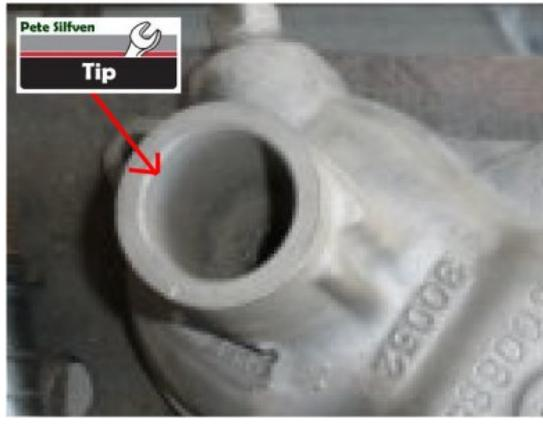
**Pete Silfven Tip:** The face of the pump housing that the seal rides on needs to be smooth and flat. If it is rusted or pitted you will need to use a facing tool to create that smooth surface, most likely at a professional shop.
