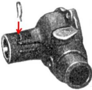
Install the bearing wire by pushing down around the groove on the bearing shaft and using kneedle nose pliers. Push down on the wire while turning the shaft will give the best results.
