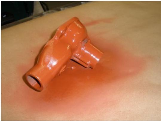
Primer the casing and the impeller.
