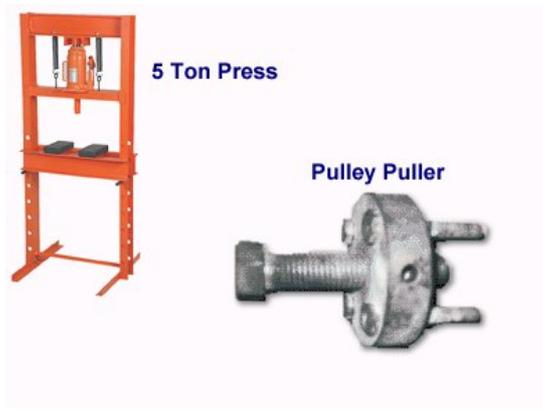
Before we start, here are they tools you will need access to. 1) at minimum a 5 ton press 2) a Pulley Puller.
