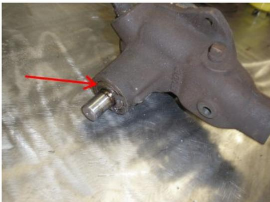
Likewise, the bearing shaft will also require a press to push the shaft out. In our case, it took a minimum of a 5 ton press to remove this bearing shaft.
