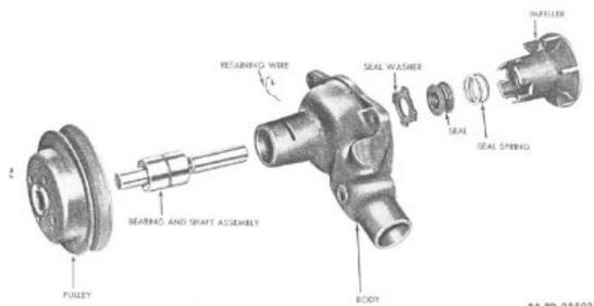
Note: you need access to specific tools to rebuild a water pump. Looking at the TM diagram of the parts for a water pump, you would think that the job would be fairly easy to accomplish. If you have specific puller and at least a 5 ton press, you will find quickly that it is not as easy as it looks.
