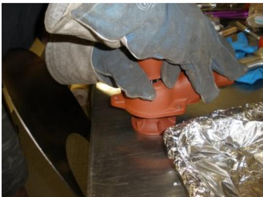
With the impeller hot, we put on some welders gloves and quickly placed the seal spring and seal on the impeller and pushed the impeller on the bearing shaft as far as we could. Then we gently tapped the top of the bearing shaft to
