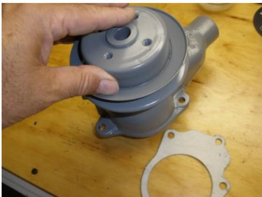
With a Cold Press, press the pulley onto the water pump shaft. You want the shaft to be right up to the edge of the pulley and you are done!
