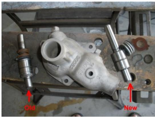
Here we have sand blasted the water pump, and compare the old bearing shaft and spring to the new rebuild kit bearing shaft. New kit looks good.
