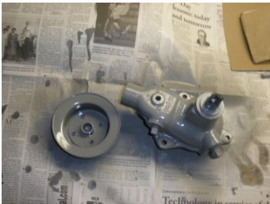
Before you install the pulley, be sure to paint it the color of your engine, OD or Gray depending on MB or GPW. Note: if you painted after the pulley is installed you would not be able to get to the underside of the pulley area.
