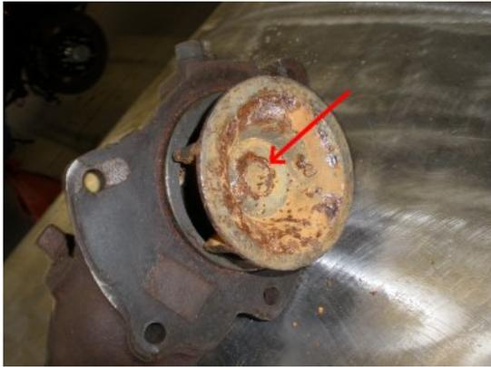
If you take a look at the cast iron impeller at the rear of the water pump, you see that the center shaft is held on by a press fit. This means to remove it you will need a press.
