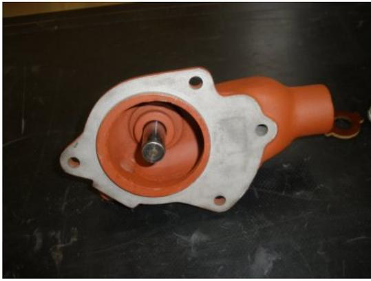
Here we take a look at the back side of the water pump bearing shaft and where the impeller will be installed.
