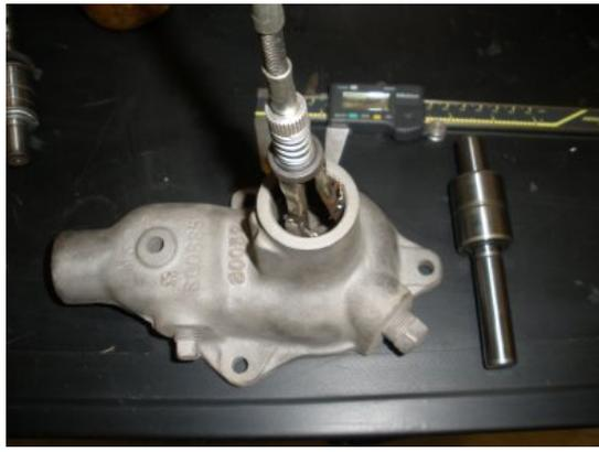
We used a standard drill and the honing kit to smooth around the inside of the water pump in preparation of the pressing the new bearing shaft.
