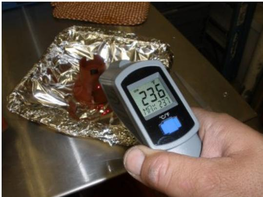
We heated the impeller for about 30 minutes at around 250 degrees. As mentioned earlier we are only a couple thousands diameter off from the bearing shaft so we want the impeller inside diameter to grow just enough for us to slap this on.
