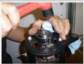
Tap the Bearings on easily. You don't want to ruin the bearing with a huge blow, so lightly tap them into position in the End Plate.
