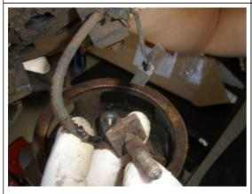
With the terminals and ground disconnected and the brushes out from their springs the cover plate is ready to come off.
