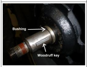
Now flip the generator over and install the bushing and woodruff key onto the commutator shaft as shown.
