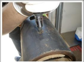
To get the field coils out, we need to use an impact wrench with a slotted end. You may need to apply a little heat and/or penetrating oil to have these brake loose. These are very stubborn to remove.
