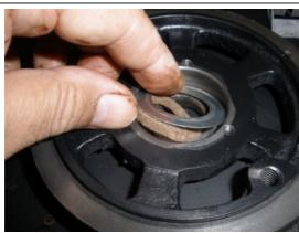
On each end of the plates, install the felt washer and reatainer ring.
