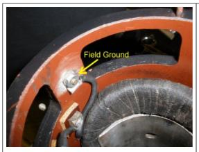
Now insert the flat head field ground screw into the outside of housing and tighten up on the inside. Here you see we have a good ground source.
