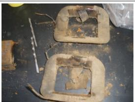
Field Coils many times rebuilders ignore the field coils. After 60 years, its time for a fresh taping. Here you see the two field coils still attached by a wire connteciton. Since the tape is practically falling off it should be replaced. You will need cloth tape and electrical tape handy.
