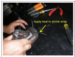
Next, we used a micro torch to quickly heat the wrap around the wire. Because the original wrap was faily thick, we used two shrink wraps around each wire by repeating this step.
