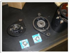
Now get your end plates, bearings, and housing to prepare to complete the reassembly.
