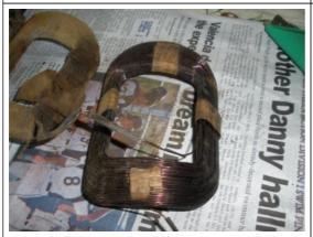
Here you see the tape is off and the four places that the paper is holding coils together. We will replace these with electrical tape. Very important not to let the coils fall out of place.
