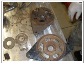
Both bearing removed, we can now send our housing out for sandblasting and start cleaning the pieces in anticipation of putting it back together.
