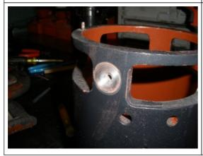
Prior to putting in your field coils, clear the paint around the ground plug, inside and out. If you don't have a good ground, your generator is not going to work. Here, we cleaned the pain around the Ground screw area. We will touch up with paint later.
