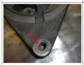
Here we are going to try and fix the generator face plate holes. Both the front and back holes have been expanded over time. In many cases, welds do not stick to cast iron..but we are going to try.
