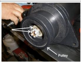
Slide the pulley over the shaft and install the shaft lock washer and castle nut as shown.
