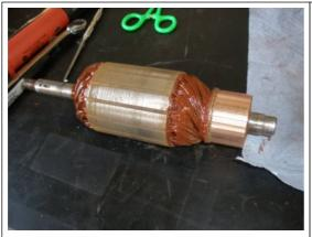
With the commutator insulating paint dried, we remove the painters tape. We hit the commutator with a little sand paper to help clean up the brass area where the brushes will ride, and the center section where the field coils are represented.
