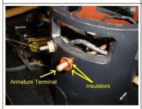
Install the insulators on the outside of the Armature Terminal as shown.
