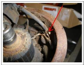
With the brushes disconntected, carefully open the faceplate so you can see the terminal connections inside the core casing.
