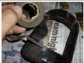
Now start wrapping the coils with the cloth tape. Again note the position of the wires so that you tape it up the same way they were before.
