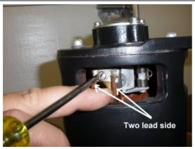
Now attach the Terminal Lead and the Brush Lead on the other side to the Spring assembly as shown. Note the position of how to screw the ends on (away from each other)
