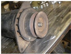
Now move the front part of the generator housing. Remove Shaft nut, Plain washer, and Lock washer
