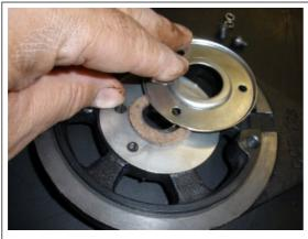
To complete the Drive End Plate, install the next felt washer and bearing retainer plate as shown
