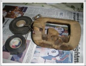
Prepare your work area by having a good roll of cloth tape as well as a roll of electrical tape. Note: if your rolls are too large you will not be able to wrap around the field coils with one piece.
