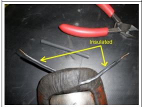
Now the wires are well insulated and we can look to repair the broken wire between the two field coils.
