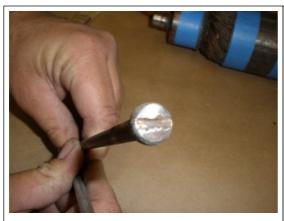
In addition, one of our long bolts need the head fixed up, so we will fill the head with a weld and cut out a new slot.
