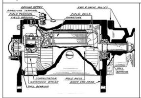
Rebuilding your generator has some challenging steps to it. Here we try to document and show you the steps to complete a rebuild. First, Let's get familiar with some of the components as shown here.
