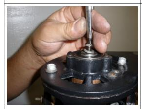
Almost done with this end. Install the Retaining washer and retainer screw into the commutator shaft
