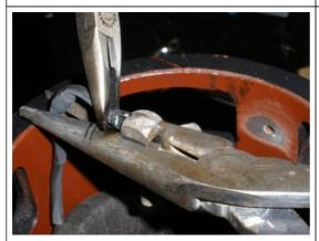
Nice, the field terminal head soldered up nicely. Now all the connectors are ready to be routed into the housing after we crank down the field coils to the housing.
