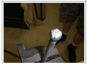
Nice new head on the long generator bolt is looking good. Ready for both bolts to be re-plated.
