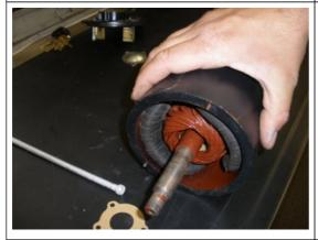
Now install the Commutator into the housing for preparation of installing the Drive End plate.
