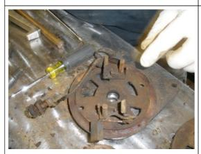
Disconnect all of the wiring on the back cover (anything with screws) leave the riveted terminals on the back.
