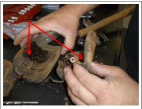
The field coils have a couple of heavy metal plates that are in the center of the field coils. You want to push those out of the center area and clean them up.
