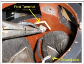
Now we are ready to install the field terminal into its slot on housing.
