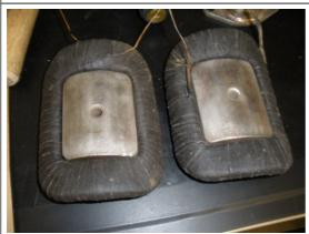
With the field coils taped, we place the cleaned field coil blocks into place. We removed the brittle insulator on the wires from the coils and will replace with new shrink wrap insulation.
