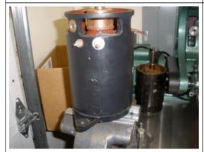
When you get the bottom plate on, turn the housing over on a vise so you can install the Commutator End Head Plate as shown.
