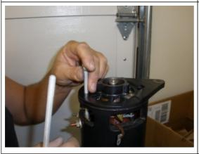
Now install the Through Bolts with lock washers into the housing.
