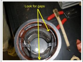
After we tighten on the field coils with the screws, we want to look for gaps to the housing. If you can see through to the other side, your field coils are not on tight enough. for the last turn, we used an impact wrench to help get it on tight enough.
