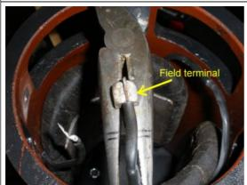
We prepared a new NOS field terminal head with solder, and now will zap the terminal head with heat and drop the wire into the field terminal head.
