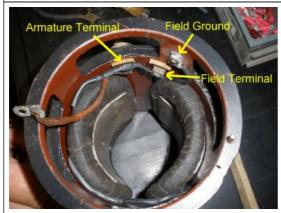
Now that everything is tightened up lets review... Both Armature and Field terminals are connected, and field ground is connected as well.
