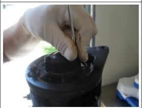
Remove the commutator cover plate screws from the back cover plate of the generator.
