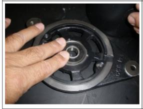
Next, install your bearings over the retainer ring. It should be a little snug, and you can tap it in gently if needed. If really tight, then apply a little assembly lube around the surface of bearing and tap in.
