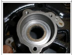
Now, install the felt washer and retainer ring the same way in the Commutator End Head Plate as shown.
