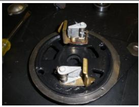
Here both brush assembly springs are installed.
