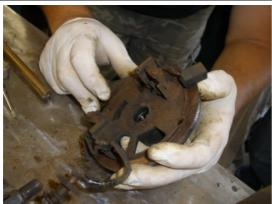
On the back plate, we need to remove the wiring that we left on from earlier.
