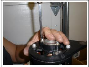
Install the cover gasket and cover plate as shown and you are complete with this end. The NOS kits have a nice plated cover plate that cleans up well from the cosmoline.
