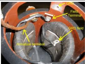
Now take the seperate Armature terminal with insulator and place it through the housing as shown. Note all the other connections around.
