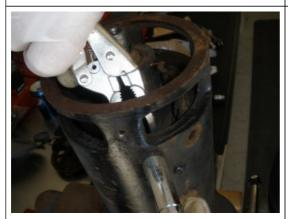
The terminals are a little difficult to get to, but you can hold one side with needle nose pliers and the other use a socket to remove the terminal nuts. Pop the terminals through to the inside.
