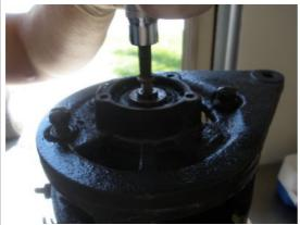
Remove the center screw from the end of the commutator end cover plate. Note: the cover plate is still connected via wiring on the inside, so don't try and pull it off yet.
