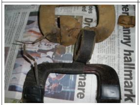
Continue taping around the coils.
