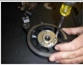
Screw in the bearing retainer plate. The NOS kits have these screws included with the kit.
