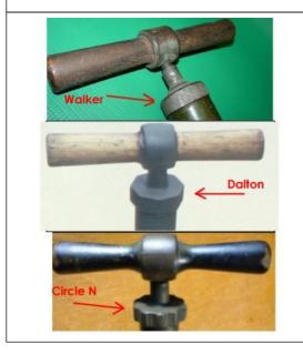
There are a couple of distinguishing features between pumps. Starting at the top of the tube. The type of cap is different among the manufactures.
