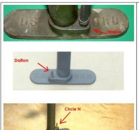
At the base of the pump there are some differences in where the valve has been positioned. Each manufacturer decided on placing the valve at a different position.
