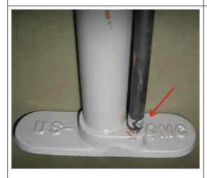
Lets first look at the Tire Pump introduction to MB's. The first tire pumps were added to the bottom of the rear seat of MB's about May of 1942 and were the QMC grey color pumps. According to Nabholtz, the QMC pumps were continued on MB's until Sept 1942. These QMC pumps did not include the Air Chuck as part of the Parts list. Part is listed as WO-A7511.
