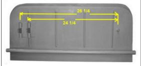
Now lets look at the air pump bracket under the rear seat. There are two possible lengths that have appeared on WWII Jeeps with a difference in the length on the bottom of the rear seat as shown. It is unclear when the differences showed up on productions lines, but most likely later in production. More research is needed to see if these sizes were both for MB's and GPW's, or just MB's.
