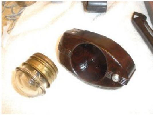
When the glass bulb pops out, you most likely will have some of the fluid all over the device from leakage. Most leak, or are short of fluid.
