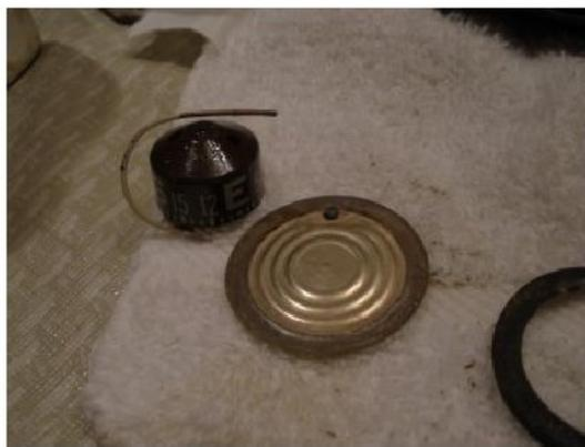
In this case you will see that the small brass "C" shaped wire broke from the back brass plate.
