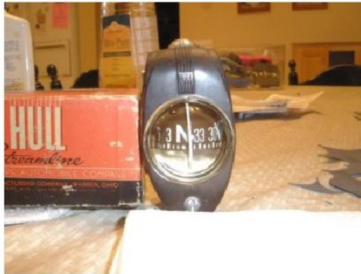
You may want to let the glass bulb sit on a paper towel for a while to see if it is leaking. If so, tighten or repeat the steps. When your done, line up the white wire vertically in the bakelite container and your done
