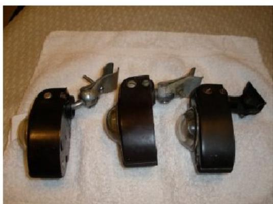
There are two different types of hinges as shown. Two which have different arms and have a clamp style and the third is mounted to a surface via screws.
