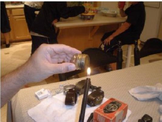
You should be able to unscrew the brass container from the glass, but these are usually frozen on there. You can heat the back and try and get it to unfreeze, Or....
