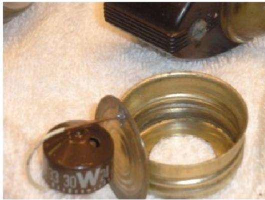
Here is a close up of the patched area. I applied the JB weld with a toothpick.
