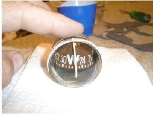
Screw the retainer on tight, and pull out of the container of lamp oil. Wipe off and you should see very little to no air in the glass bulb
