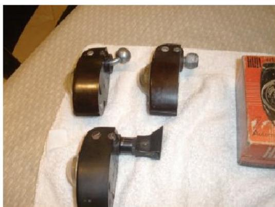
Turning these on their sides you can see a few differences. The arms that hold the compass to a Windshield or Dash, and two the screws to dismantle the magnets for the N-S and E-W screws
