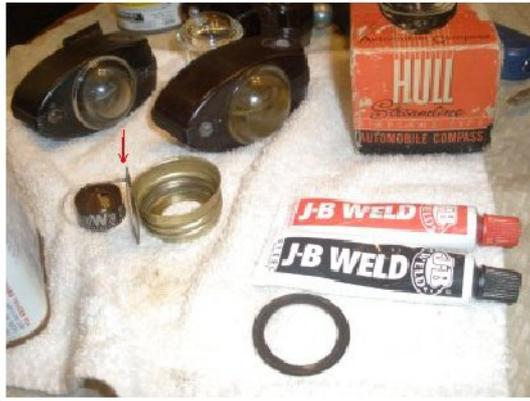
To fix the wire to the back plate I used JB weld. I like this product and it will withstand heat and the keroscene lamp oil I will be filling later, so I applied the JB Weld and let it sit overnight.
