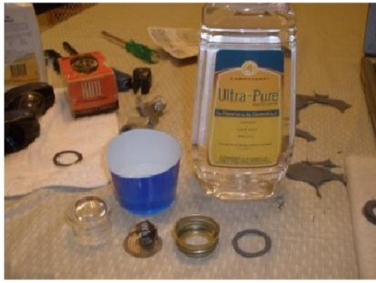
Now that the fix is made to the compass and the gasket is ready, I pour the non odor pure lamp oil into a cup I cut in half. I will submerge the entire glass bulb to remove as much air as possible.
