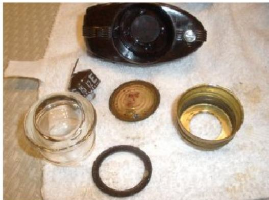
After a little time soaking in the penetrating oil, you will find that the two brass fittings will break free and you can see all of your pieces. Dump out the fluid and clean the glass.
