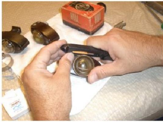
To remove the glass bulb can be done a couple of different ways. Use some sort of a knife to get underneath the glass lip and pull upward. Be careful not to damage the glass or the holder. Bulb should pop right out.
