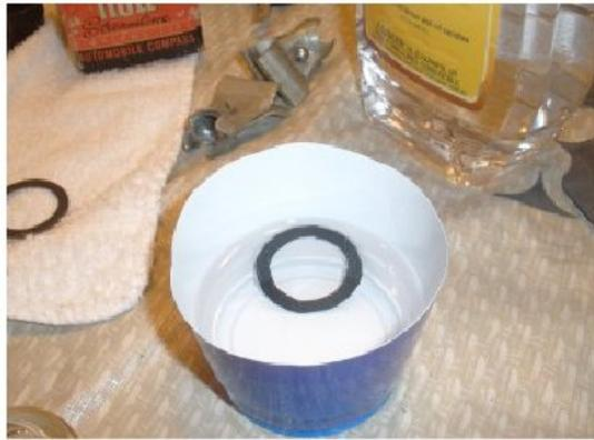
Prior to putting the items together, I soak the new gasket in the lamp oil to get it saturated. This will help when I place the items back together.
