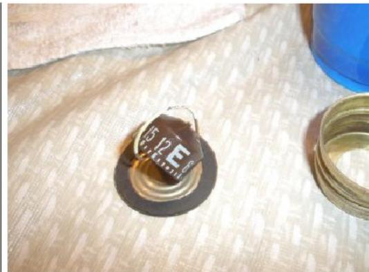
After saturating the gasket, I place it around the back plate to make sure the fit will be good
