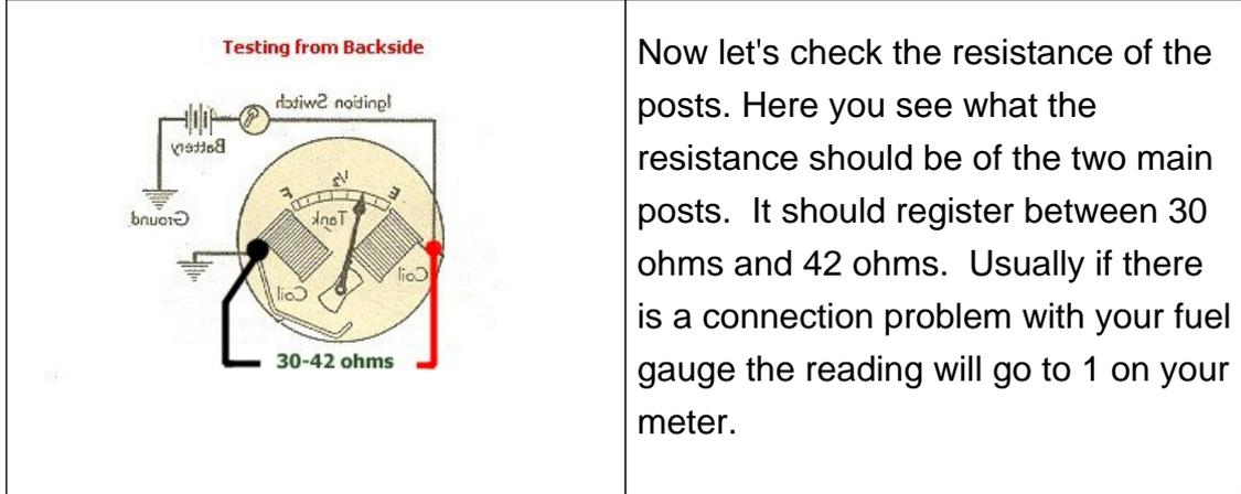
Now let's check the resistance of the posts. Here you see what the resistance should be of the two main posts. It should register between 30 ohms and 42 ohms. Usually if there is a connection problem with your fuel gauge the reading will go to 1 on your meter.
