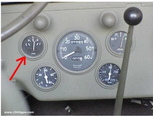
Now install the Fuel Gauge and hook up the connections. When the ignition is OFF, the Fuel reading should be sitting on EMPTY. If you turn on the ignition and the fuel gauge JUMPS to FULL (and the tank is not full) then most likely there is an issue with the Sending Unit. If it reads correctly then your set!
