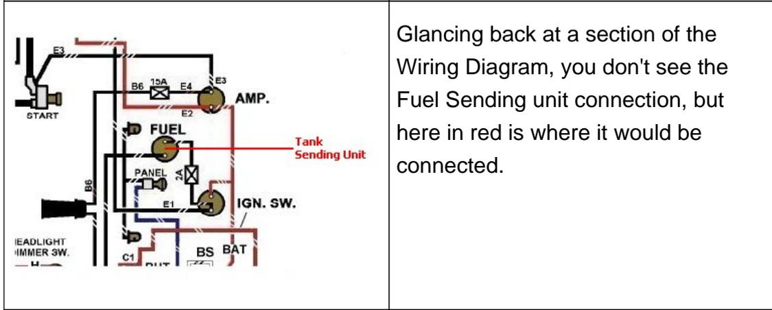
Glancing back at a section of the Wiring Diagram, you don't see the Fuel Sending unit connection, but here in red is where it would be connected.
