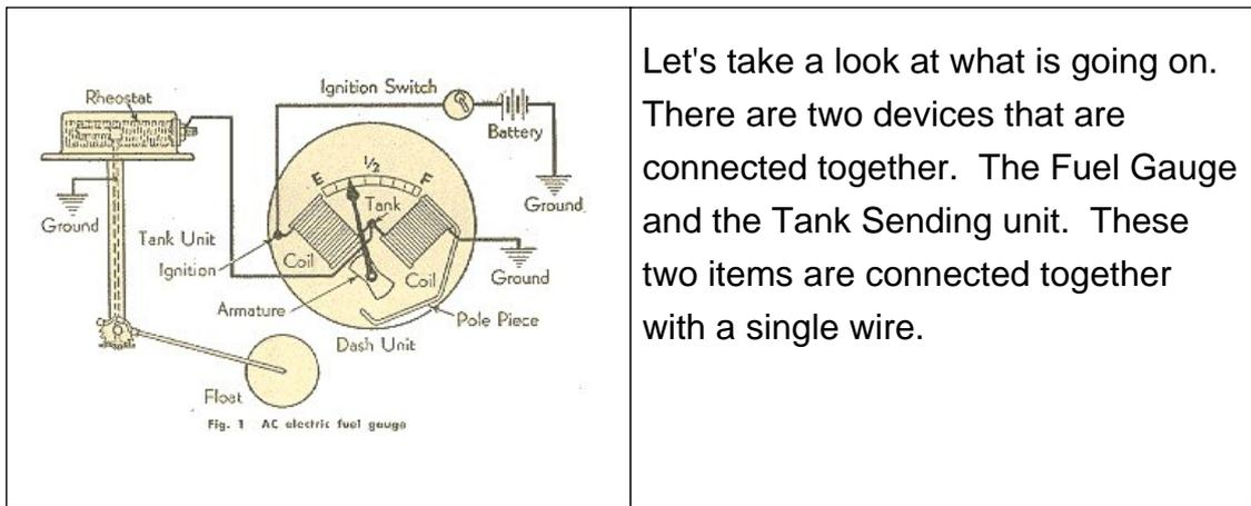
Let's take a look at what is going on. There are two devices that are connected together. The Fuel Gauge and the Tank Sending unit. These two items are connected together with a single wire.
