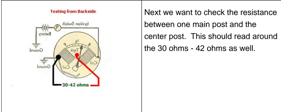
Next we want to check the resistance between one main post and the center post. This should read around the 30 ohms - 42 ohms as well.
