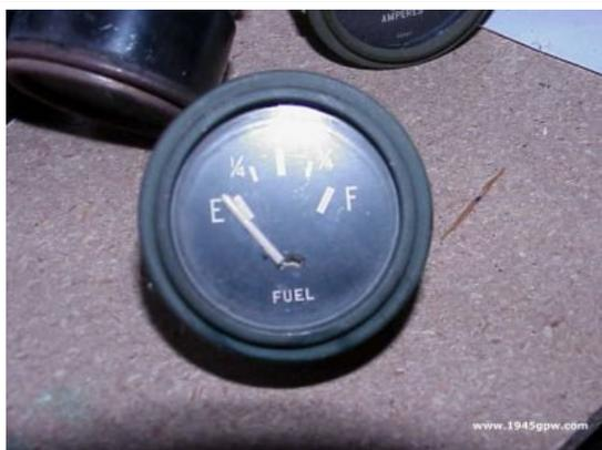
The Fuel Gauge in the 40's is built on electrical resistance. The more resistance from one post to the other allows the gauge to move from one side to the other. Nine times out of Ten the problem with a Fuel Gauge reading has to do with the grounding on the gauge.
