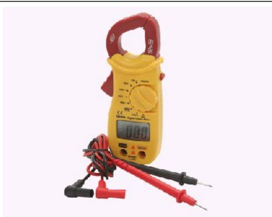
You will need a simple meter to test the ohms on your fuel gauge. These are really inexpensive currently. This one was \$9.99 at Harbor Freight. These are necessary to troubleshoot electrical problems with your jeep.
