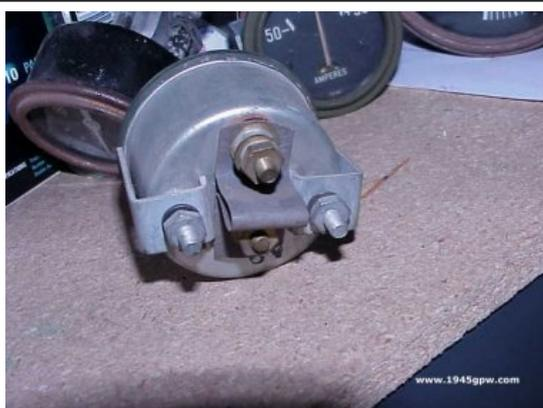
If your fuel gauge doesn't work while in your jeep, pull it out and you will need to get a meter and check the resistance of the posts on the back side of the gauge. One post is for the power from the ignition, the middle post is the connection from the Fuel tank sending unit, and the last post is for a ground.
