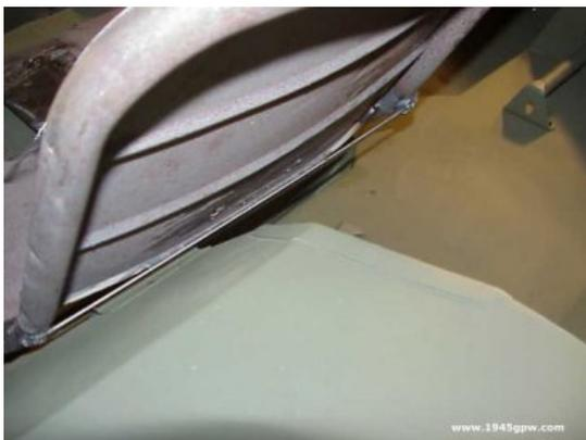
Her you see it sits on the wheel well nicely. If you look closely, you can see where the hole in the wheel well will have a bolt that will connect to the back of the flat bar and keep the flat bar on the support of the wheel well. Looking good.
