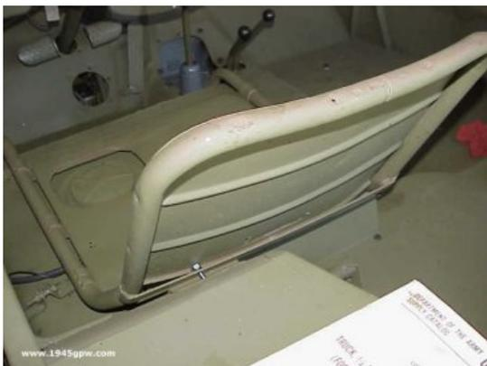
I marked the location that I needed to drill from the hole in the wheel well. I pulled the chair back out and drilled the hole as needed. Next, I put tank cover plate on (back of the driver seat, and then installed the chair, I tightened everything up and it looks good.
