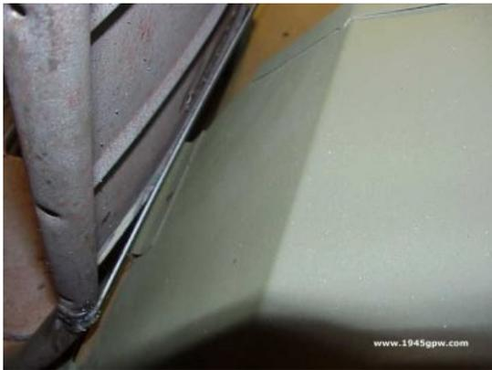
Another angle to look at... note, the flat bar will need to bow out a bit to sit on the wheel well nicely... we will resolve that when we tack in the passenger side of the flat bar.
