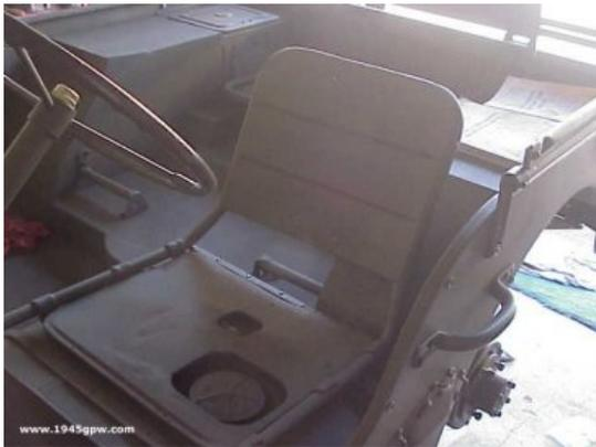
Now that the chair is painted, I bolted in the front two bolts to the chair so I can mark and drill the hole in the back brace that connects to the wheel well.
