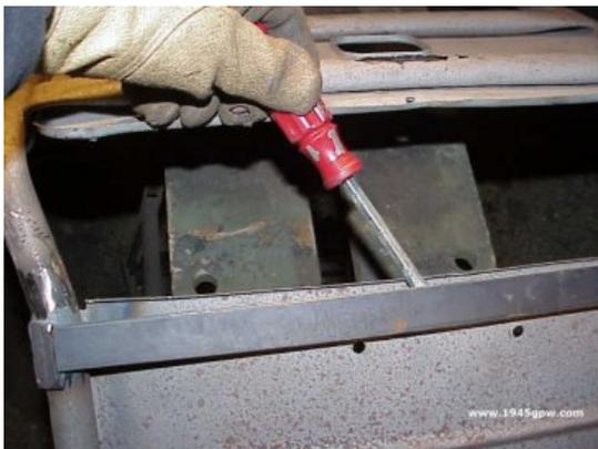
Now, we want a little "bow" in the bar to sit on the wheel well, so cut the flat bar a little long. Here you see I pried the flat bar out so it would fit on the passenger side and give it about 1/8in bow, and is tight.
