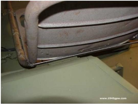
Before tacking in the passenger side, I wanted to look at the position to make sure it would land on the wheel well properly. I was looking to make sure the seat would be above the gas tank, and that it would sit on the wheel well for support. It does... so I can continue
