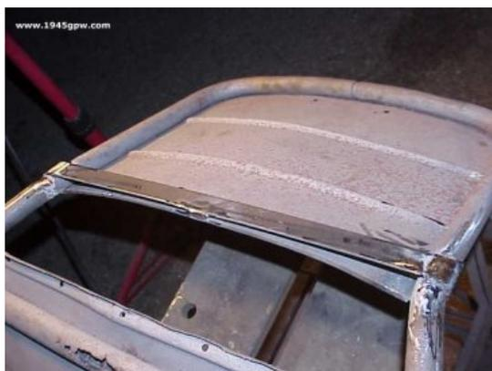
Here I finished welding the flat bar in. I also tacked in, for support a little section in the center to the back of the seat for additional strength.
