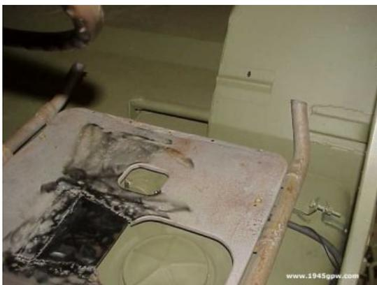
I cut the chair at the angle of bend that would go right up the wheel well. After this cut, I placed the seat back in the jeep to take a look at the angle of the seat. It looked good, so now I will shave off a little of the top of the chair to continue the angle and tack the chair back together and verify.
