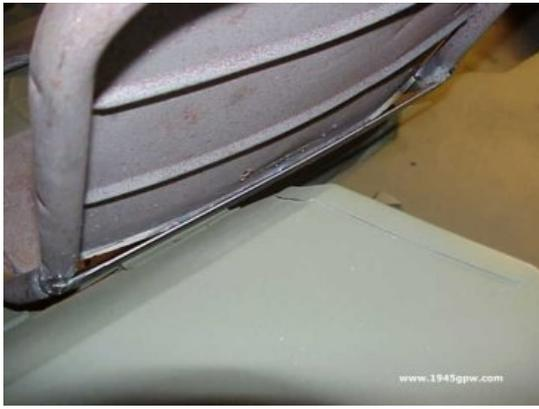
The final fit looks good. Now I need to fill some holes in the seat, drill the hole from the wheel well, and fit a nut behind the flat bar (original tube had a caged nut)... primer, paint and cover.
