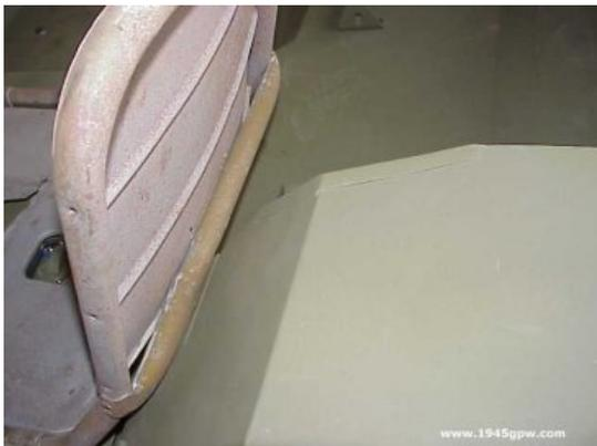
The Driver Seat modification is pretty basic that anyone to do, and do in different ways. The basic idea, is to remove the round tube on the back support which takes up to 2-3in forcing your back forward. We want to utilize this room, but removing the round tube, bending the chair to incline more, and replace it with a flat bar for support. That simple.
