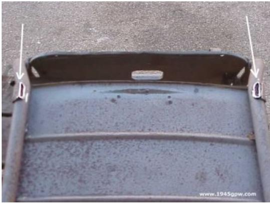
The first part of the modification is to remove the tube from behind the seat. You're going to shave off a little more on the driver side than the passenger side when the flat bar gets measured up. Start with this and you can adjust a little later. After you do this, place the chair back into your jeep and you can see how much room you have to bend.
