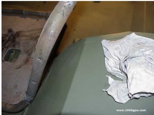
After tacking the two pieces back together, I set the chair back in the jeep to verify the angle. Notice how it has given be me a good 3-4in now because of the incline. I am content with the angle, so I will firm up the welding, and grind it up to look good.
