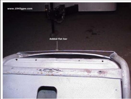
Here you can see the flat bar bowing out. This will work great sitting on the wheel well. So time to tack the flat bar in and check the fitting in the jeep.
