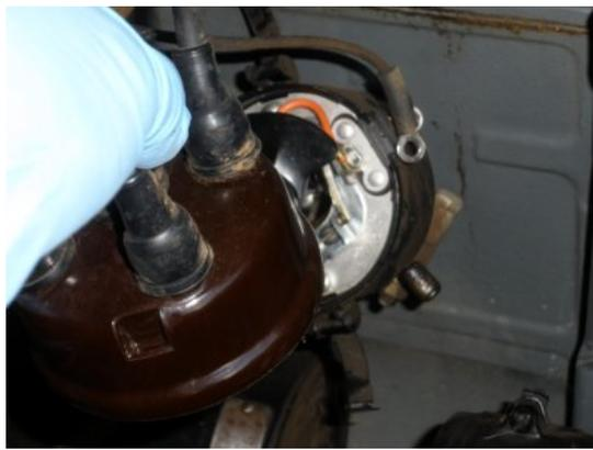
Remove the distributor cap from the distributor. Move it out of the way as we will be pulling the distributor out.
