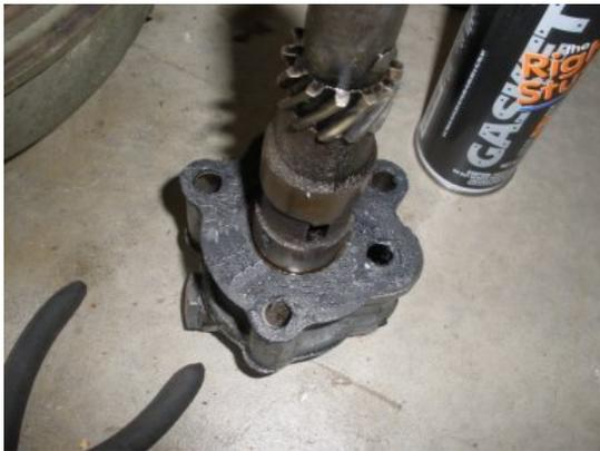
Note: The offset of the oil pump and the distributor need to line up correctly for this to work. Don't assume that it will line up. Before applying sealer, make sure the rotor and oiler on distributor are in the correct position. If you are certain it looks good...
