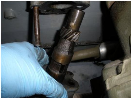
To disengage the gears on the oil pump from the cam shaft, you will need to pull the oil pump downwards. Note: oil pump will have oil in it.
