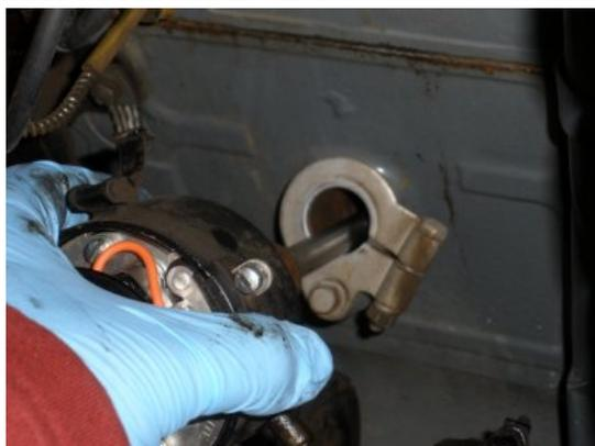
Once the distributor connection is loosened, you can pull the distributor out of the block.
