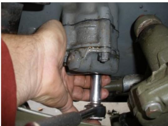
Now, insert your distributor shaft back into the block and engage it back into position with the oil pump shaft. The distributor now should be in an approximate position for the time and the TDC of piston #1
