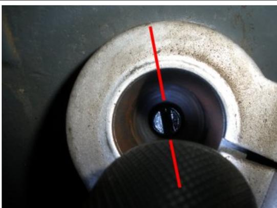
Look down the hole for the distributor on the block and see if it is going to be pretty close to your expectation. Reminder: The teeth of the gear will move your desired position more towards a counter clockwise position. You may need to turn the gear back one or two teeth to line up correctly.
