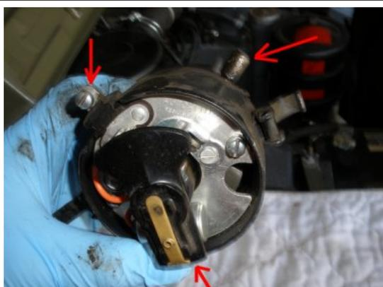
While the distributor is in your hand, rotate the distributor casing so that the oiler is about the 2 o'clock position and while holding the casing, rotate the rotor to just shy of the 6 o'clock position.. This is close to the proper positioning.
