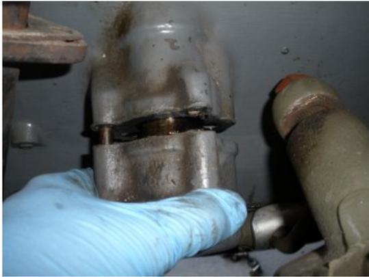
Note: there are two sections from your oil pump to separate, a lower section versus the upper section. You want the upper section to separate.
