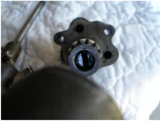
After turning the gear on the oil pump (in the position that you would bolt it in) but bring it back about two teeth back (as the spin of the gear will take it to the right), you see that the oil pump is in the approximate position to receive the Distributor shaft.
