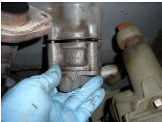
Next, re-engage the oil pump into the position that you have turned the gear to. Do not bolt in yet, we need to see if it is in the correct position.
