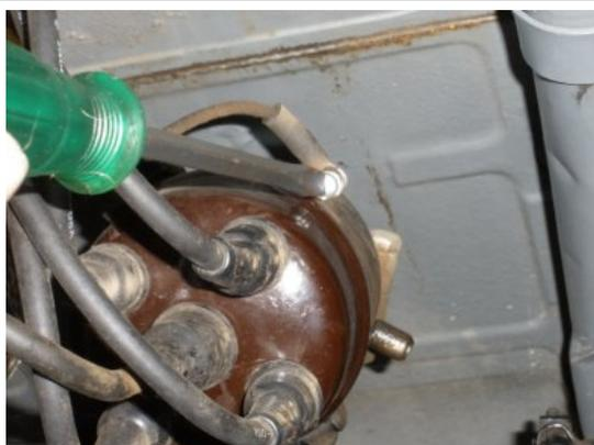
You will be working on boths sides of the engine, and Note: your TIMING will be effected. So be prepared to time your engine at the end of this article. First, disconnect the coil wire from the distributor.
