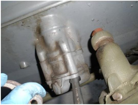
Remove the bolts on the oil pump on the opposite side of the engine. You will need to tug a little as the gears will disengage from the camshaft as there is probably sealer on the gaskets.
