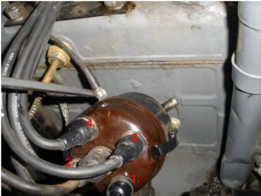
Replace the wire from the coil to the distributor (should fit better). Check your wires to make sure they are still in 1-3-4-2 order on your distributor cap.
