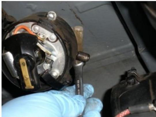
Loosen the connection for the distributor to the engine block.
