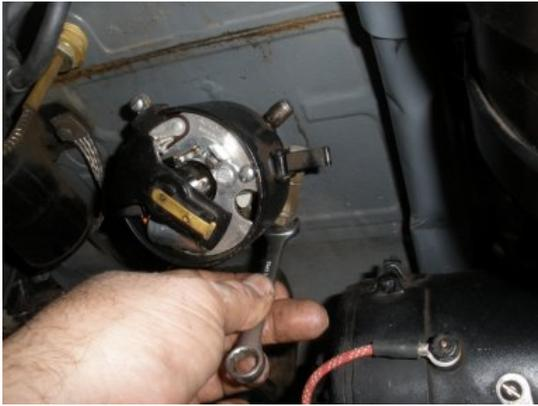
Slightly tighten the distributor shaft to the block, and clamp the distributor cap back on the distributor.
