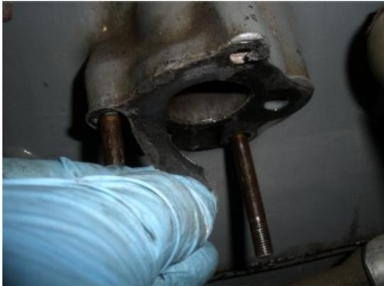
Remove the old gasket from the block and oil pump. Note: Prepare your oil pump to be re-engaged and replace the gasket. Clean the surface on the oil pump as well.
