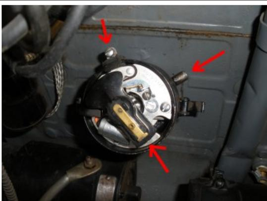
Slightly tighten the distributor shaft into position. It should be loose enough to turn the distributor for timing later.
