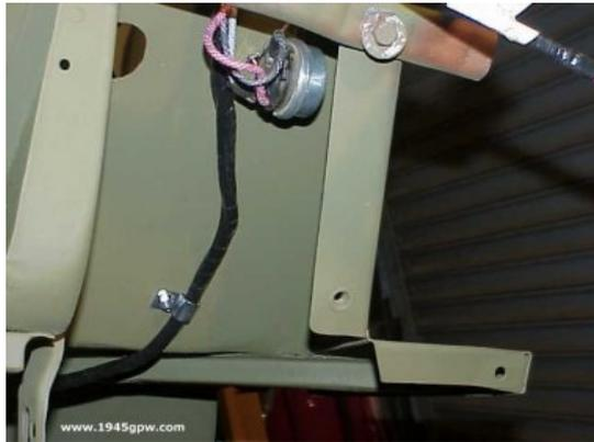
Follow your main cables back to the front of the jeep and wire up the headlight foot dimmer switch pulling the excess main harness towards the front. Add clip to hold harness in place.
