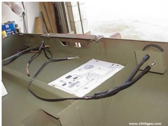
Here the tail lights wiring is laid out with the tub upside down. After the connectors have been attached to the tail lights you can easily see from the diagram where the wires are connected.
