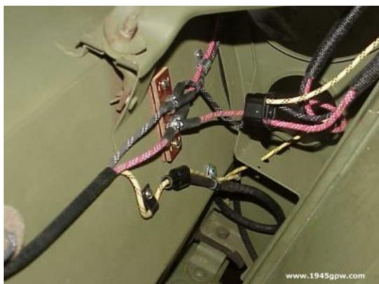
Now install the wiring to the small junction for the headlights and the black out lights. Similar connections as you saw with the tail lights. Snap each of the connections together, and wrap up with electrical tape.
