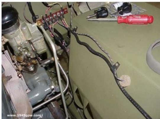
Now run the wiring for the headlights from the Main Junction. You should have two sections one for the headlights and one for the black out lights. Review the diagram and lay the wiring lengths out into position.
