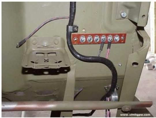
Assuming that your tub is in a rotisserie, Install your main junction block on your firewall. Next, stretch out your Main Wiring Harness and connect the black and red wires to the junction block. This will be your starting point.
