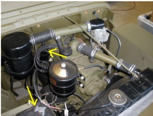
And last, (Early models) connect your wires from filterette, and junction, then connect your Coil wiring as per the wiring diagram and your battery... you should be ready to go!!
