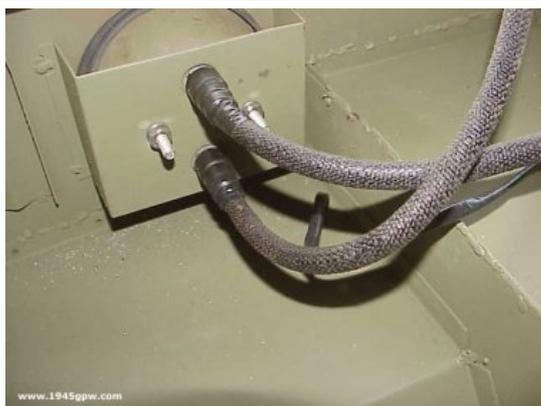
After you have the tail lights connected, inspect and use some electrical tape to cover your connections from your main harness to your tail light wires. Note: on the driverside you should have the trailer socket wiring that will go up into the tool box.
