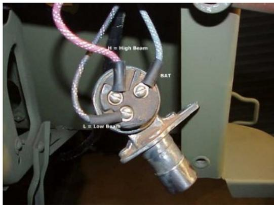
Next follow the main harness down from the junction block and install the wires to the Headlight Dimmer switch. Once you connect the wires, install the dimmer switch onto the tub.
