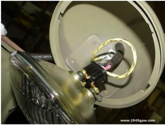
Run the wires into each of the two head light buckets, and wire up as shown on the wiring diagram. Follow the wires for the front black out lights as well.
